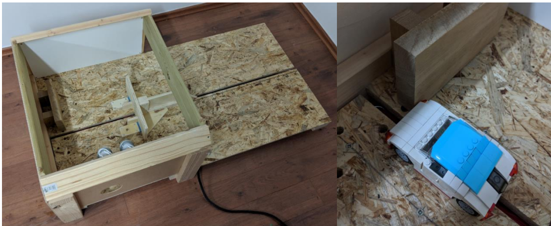
Figure 10: crash sled (left) and positioned car for 25% overlap frontal crash (right)
