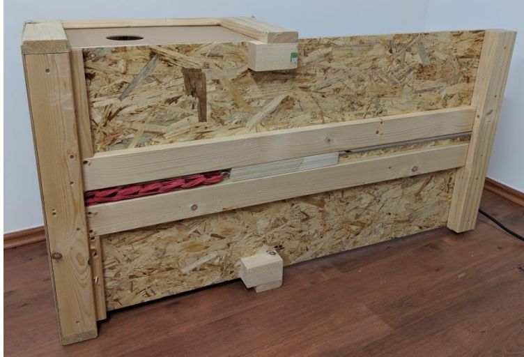
Figure 11: crash sled from below with slingshot mechanism
