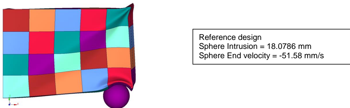
Fig.4: Results of the finite element simulation of cantilever frame hit by a rigid sphere
