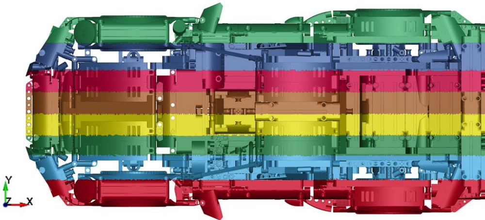
Fig. 14: Domain decomposition for simulation with 8 CPUs.
