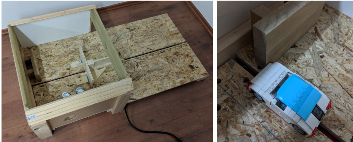
Fig. 15: Crash sled (left) and positioned car for 25% overlap frontal crash (right).
